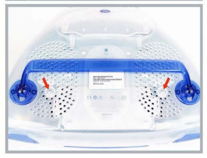
Place the iMac on a safe surface, carefully turn it upside down and remove the two screws near the front stand.
