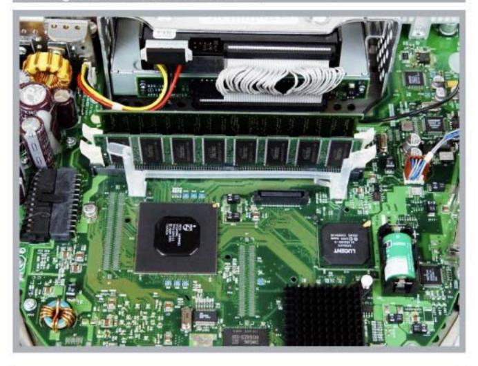
Remove the installed memory by spreading the white tabs, and lifting straight up. Be careful to not touch the contacts. Store the memory in a safe location, preferably an antistatic bag.
