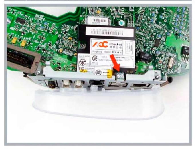
Carefully turn the logic board aver and remove the LAST screw!
