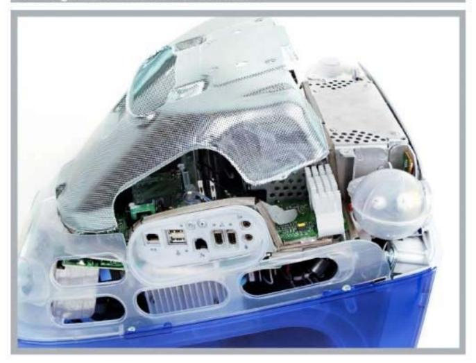
Remove the steel cage being extra careful of the sharp edges.
