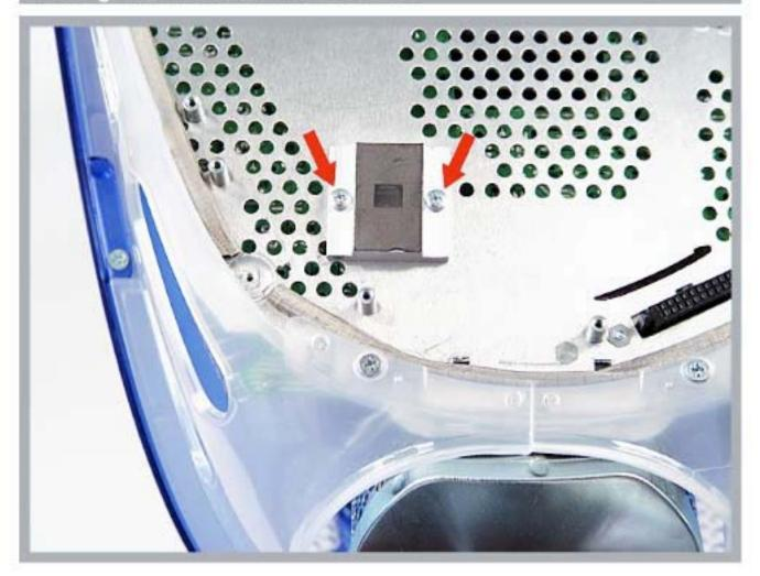
Remove the heat sink from the iMac. It will be replaced be another heat sink supplied by us. As always, save your screws.
