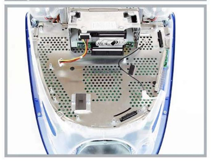
With all the screws removed, the logic board can easily be removed from the iMac. Set it carefully on the large anti-static bag provided.
