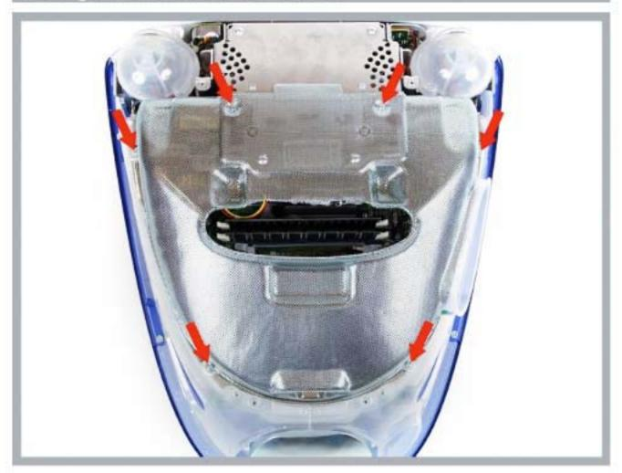
Guess what? More screws. Remove the six steel cage screws with the supplied magnetic screwdriver, being especially careful to not let them fall into the iMac.
